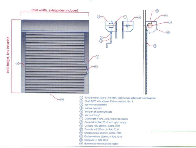
All outer parts of the shutter are aluminium, coated in RAL 7016.
